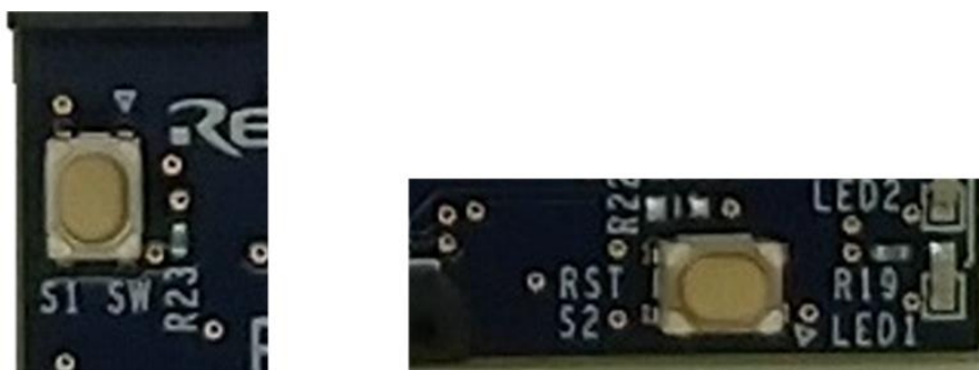
Figure 17. Reset Switch (S2) and User Switch (S1)
