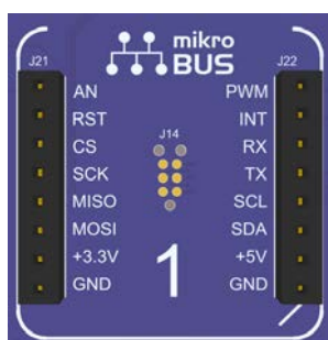
Figure 14. mikroBUS Connection
