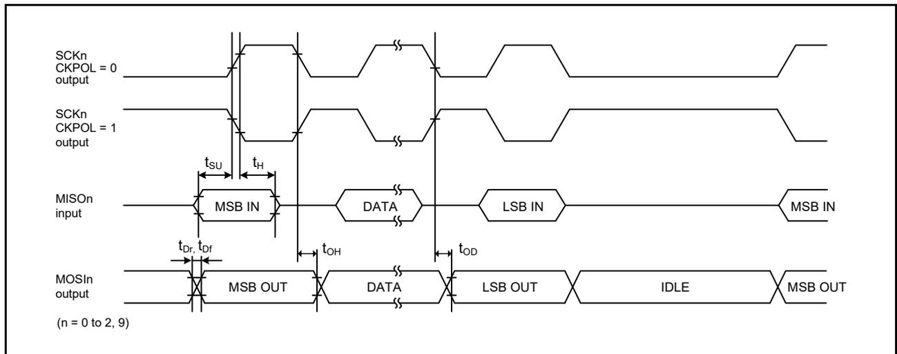
**Figure 2.47 SCI simple SPI mode timing for master when CKPH = 1**
