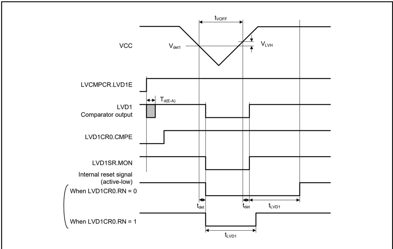
Figure 2.76 Voltage detection circuit timing ( $V_{det1}$ )
