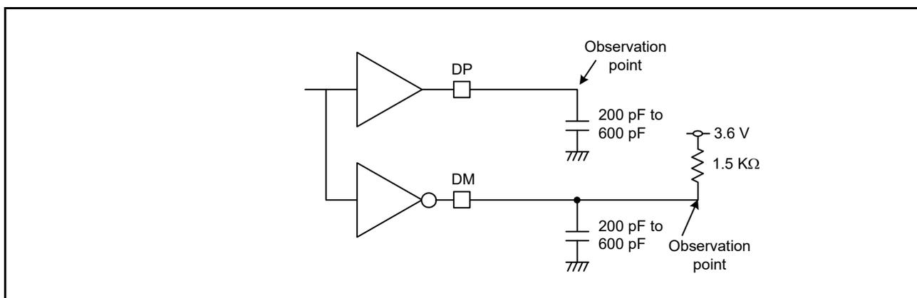
Figure 2.67 Test circuit for Low-Speed (LS) connection
