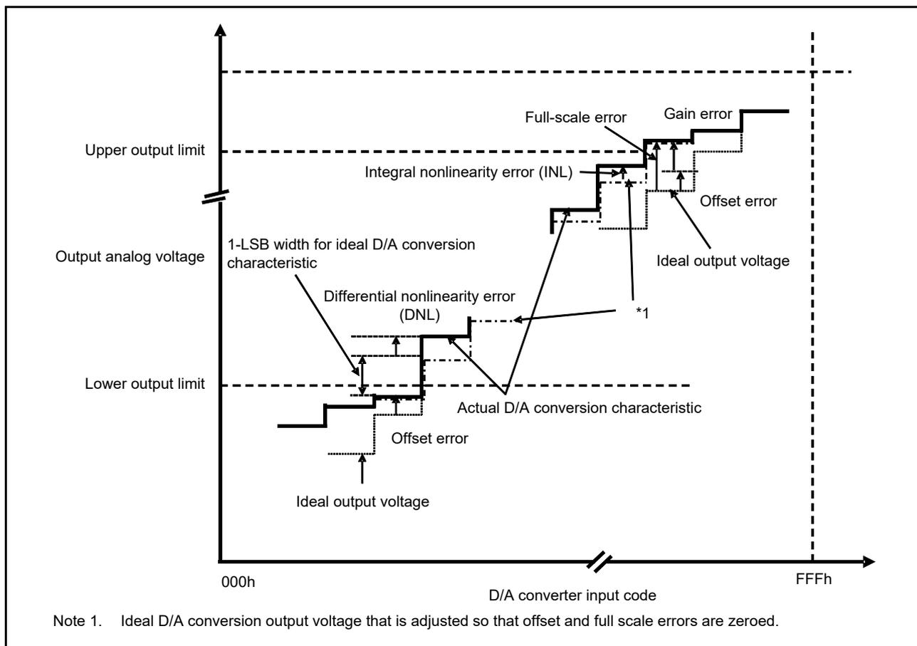
Figure 2.71 Illustration of D/A converter characteristic terms
