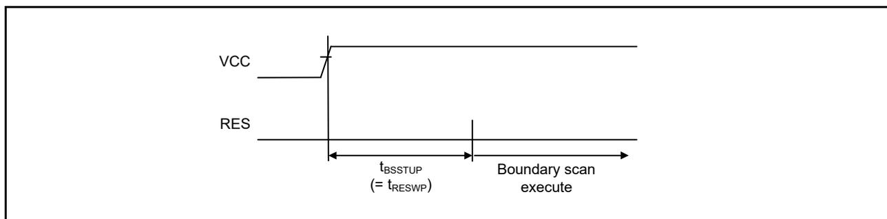
Figure 2.84 Boundary scan circuit start up timing
