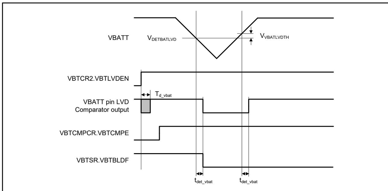
Figure 2.80 VBATT pin voltage detection circuit timing
