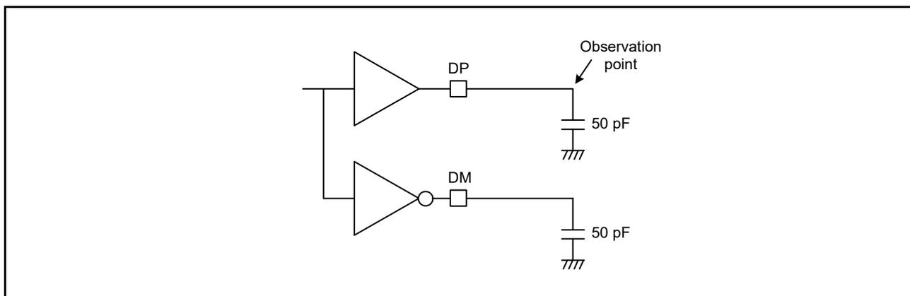
Figure 2.66 Test circuit for Full-Speed (FS) connection
