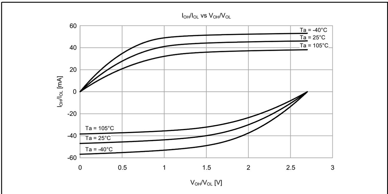
Figure 2.13 V<sub>OH/V<sub>OL</sub></sub> and I<sub>OH/I<sub>OL</sub></sub> temperature characteristics at VCC = 2.7 V when middle drive output is selected (reference data)
