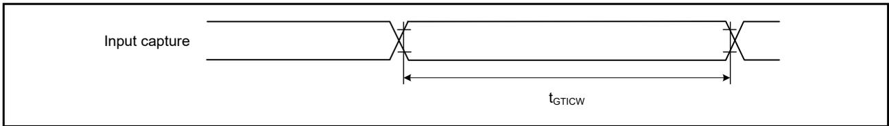
Figure 2.40 GPT input capture timing
