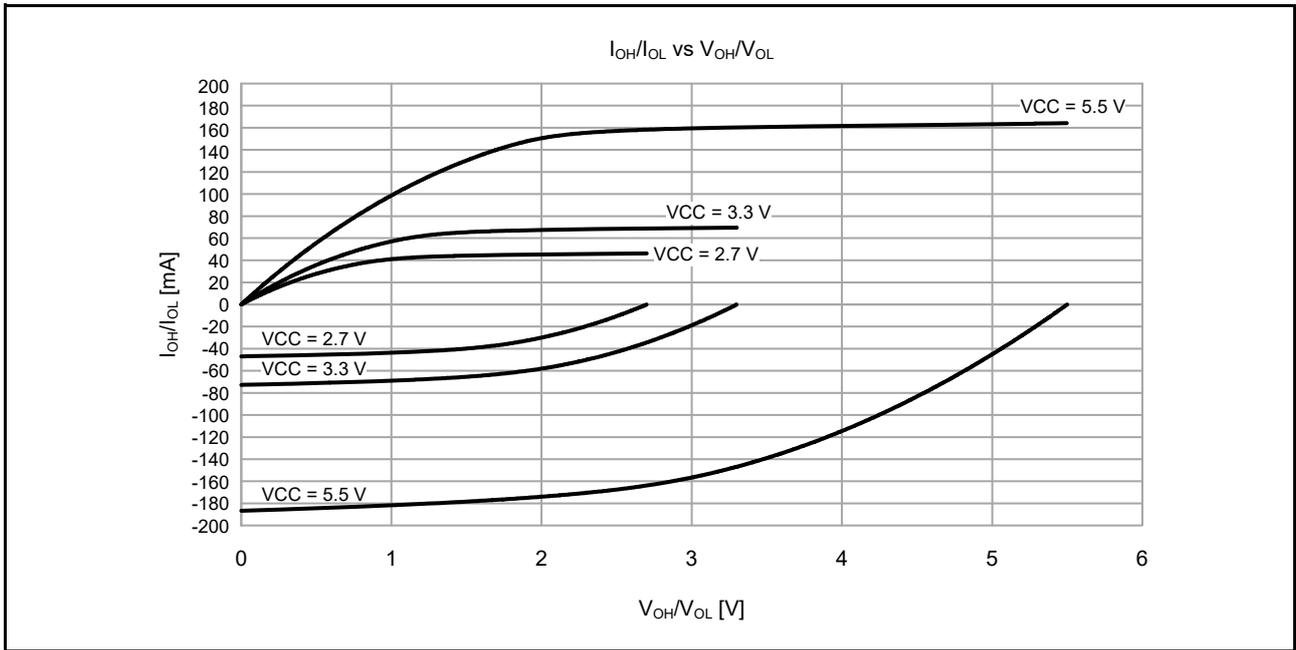
Figure 2.12 V<sub>OH/V<sub>OL</sub></sub> and I<sub>OH/I<sub>OL</sub></sub> voltage characteristics at Ta = 25°C when middle drive output is selected (reference data)
