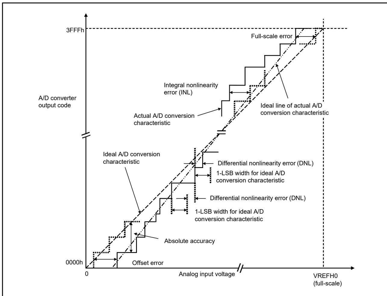
Figure 2.70 Illustration of 14-bit A/D converter characteristic terms
