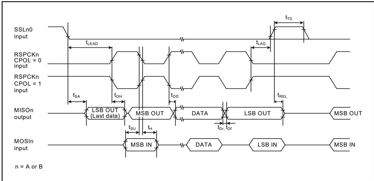
Figure 2.58 SPI timing for slave when CPHA = 1
