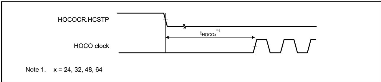
Figure 2.27 HOCO clock oscillator start timing (started by setting HOCOCR.HCSTP bit)
