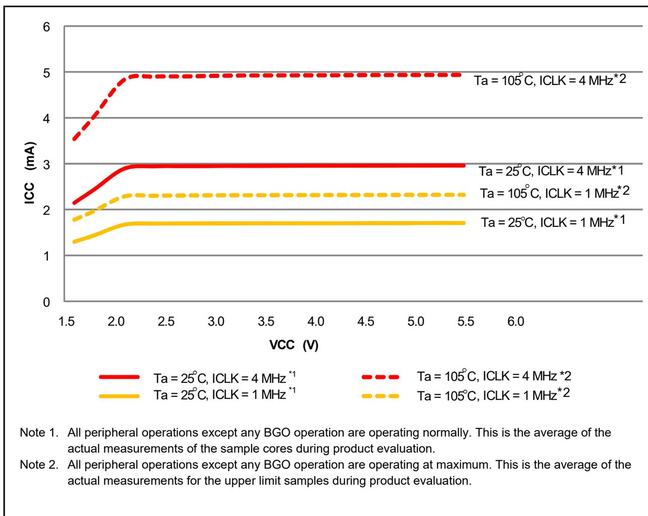
Figure 2.20 Voltage dependency in low-voltage mode (reference data)
