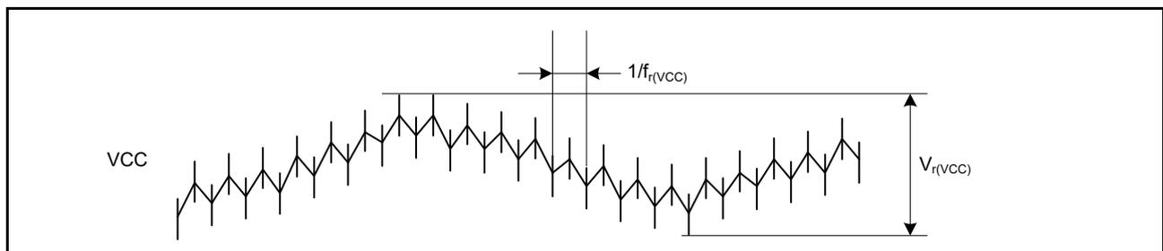
**Figure 2.24 Ripple waveform**
