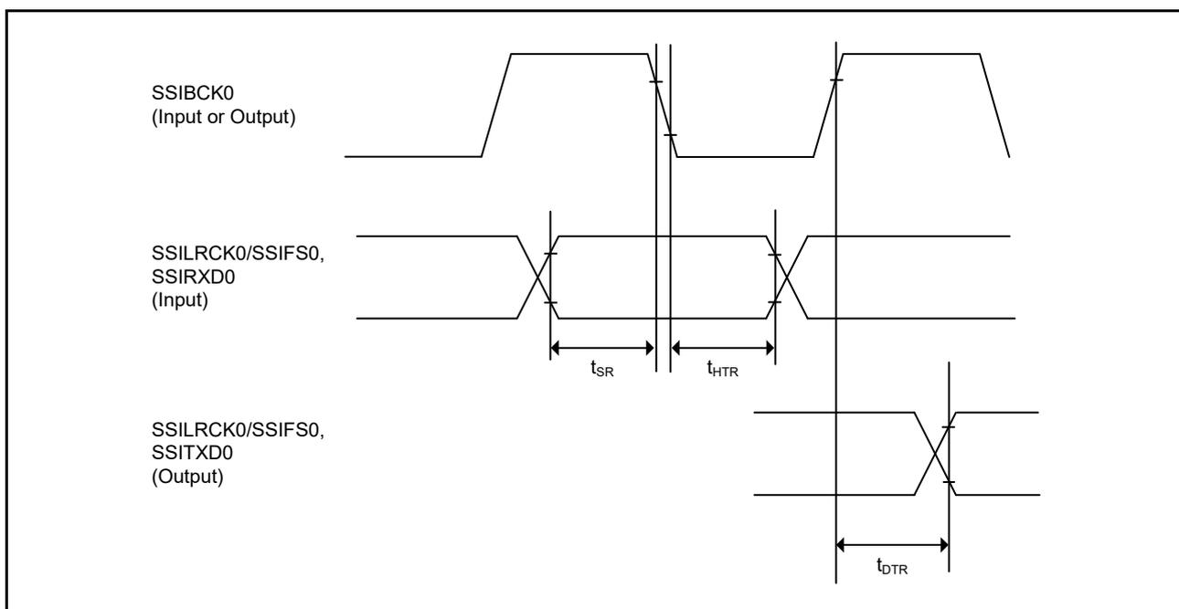
Figure 2.62 SSIE data transmit/receive timing (SSICR.BCKP = 1)
