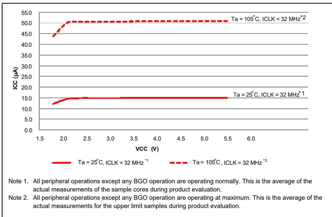
Figure 2.21 Voltage dependency in Subosc-speed mode (reference data)
