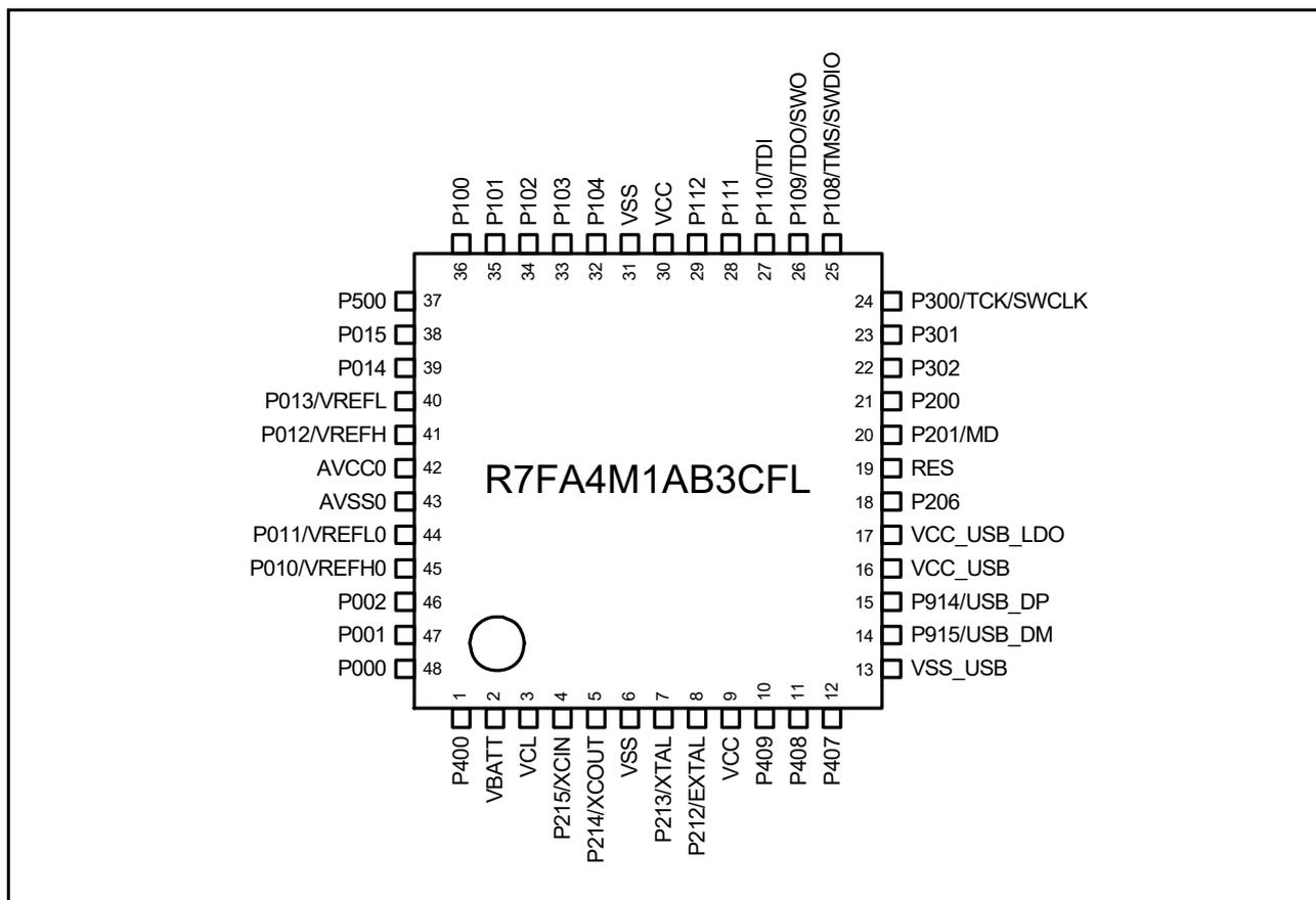
Figure 1.7 Pin assignment for 48-pin LQFP (top view)
