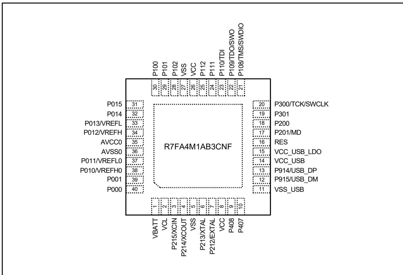
Figure 1.9 Pin assignment for 40-pin QFN (top view)
