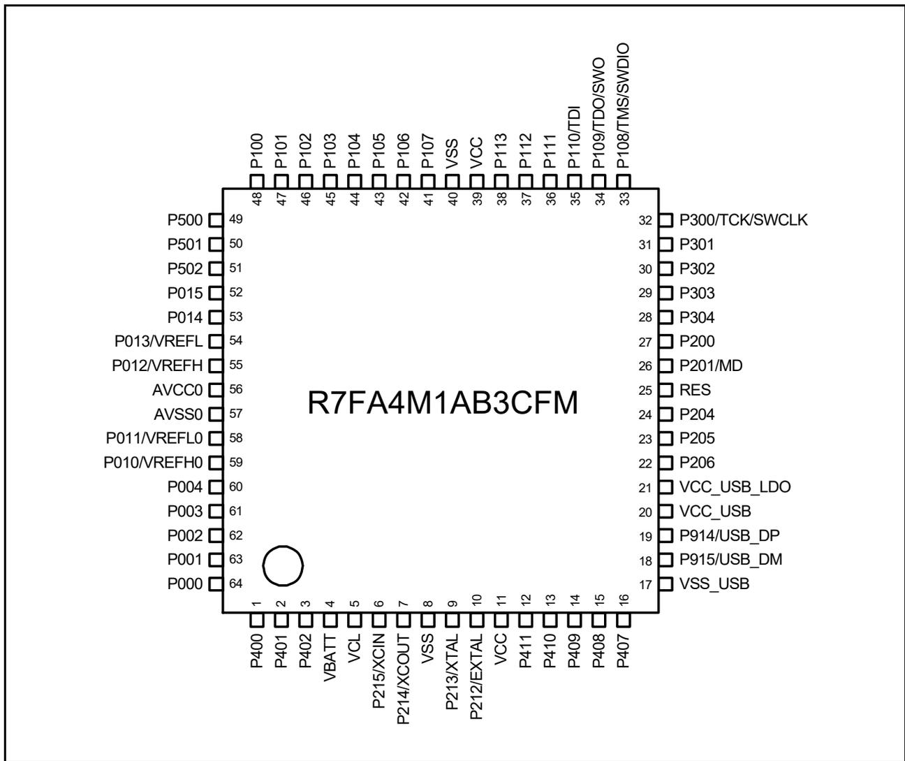
Figure 1.5 Pin assignment for 64-pin LQFP (top view)
