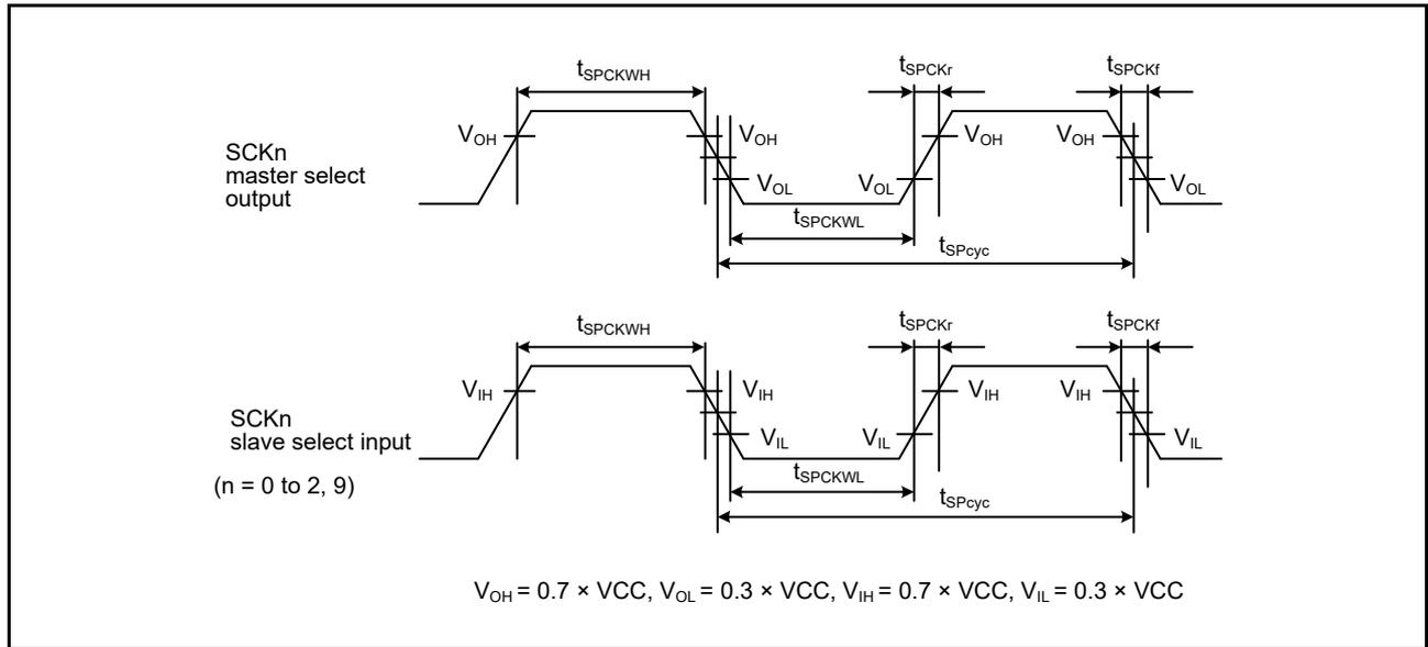
**Figure 2.46 SCI simple SPI mode clock timing**
