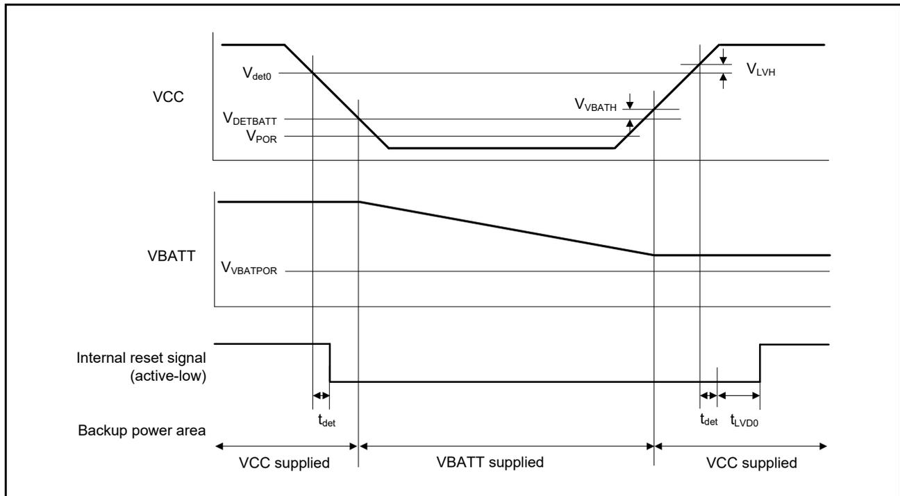
**Figure 2.78 Power supply switching and LVD0 reset timing**
