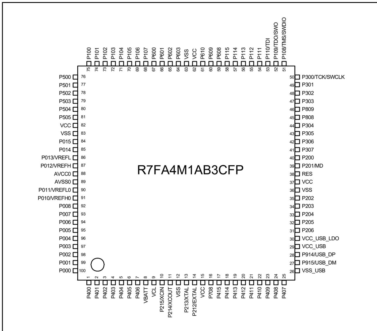
Figure 1.3 Pin assignment for 100-pin LQFP (top view)
