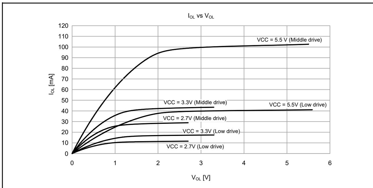
Figure 2.16 V<sub>OH</sub>/V<sub>OL</sub> and I<sub>OH</sub>/I<sub>OL</sub> voltage characteristics at Ta = 25°C
