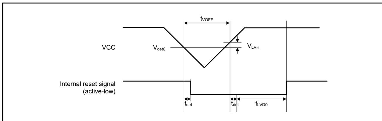
Figure 2.75 Voltage detection circuit timing ( $V_{det0}$ )
