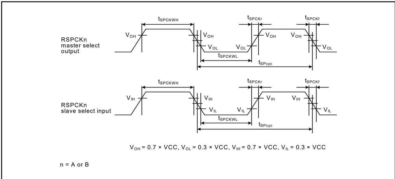
Figure 2.52 SPI clock timing
