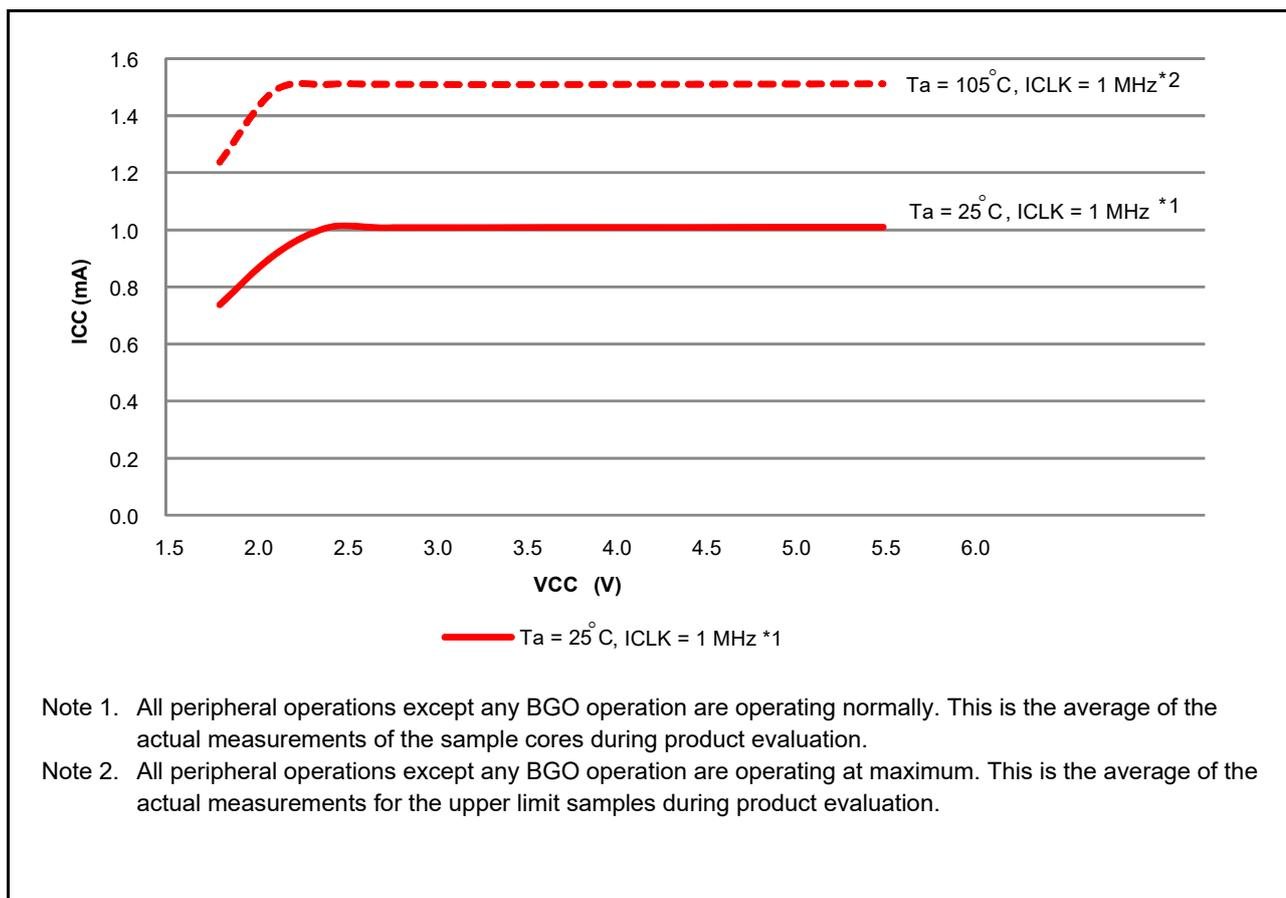
Figure 2.19 Voltage dependency in Low-speed mode (reference data)
