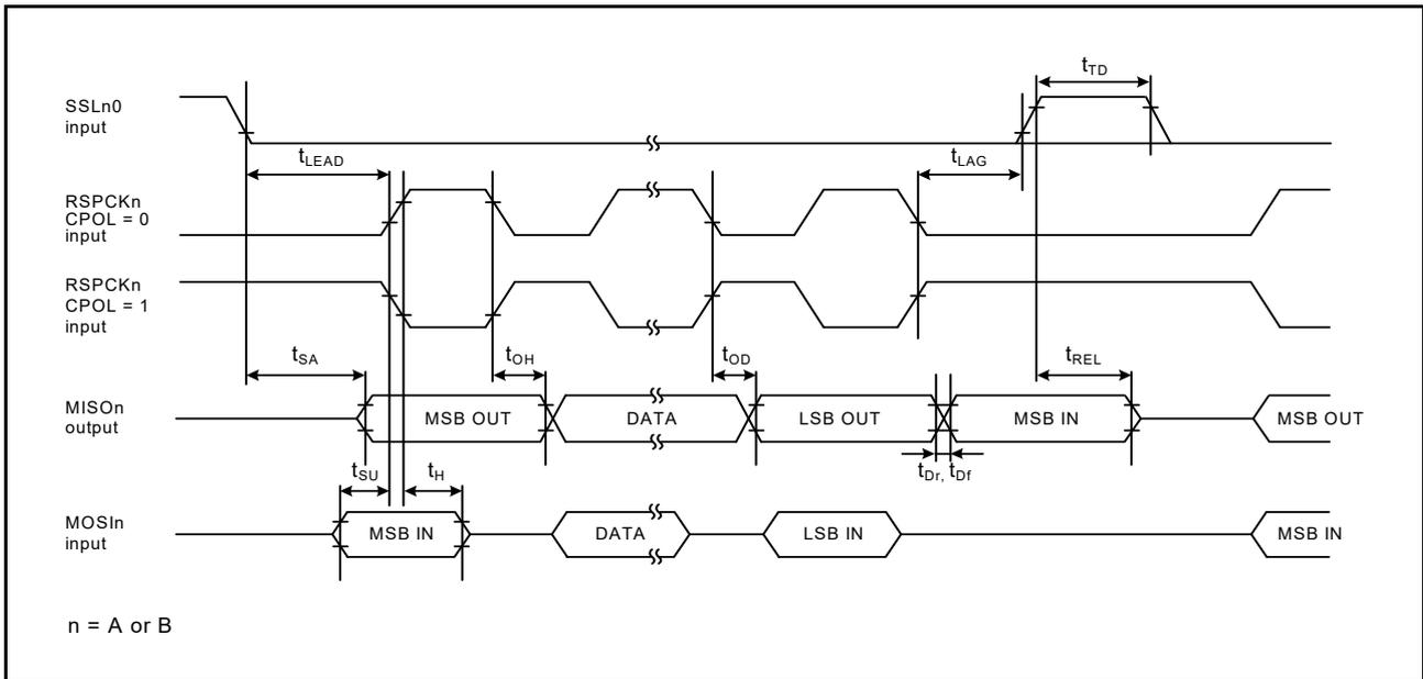
Figure 2.57 SPI timing for slave when CPHA = 0
