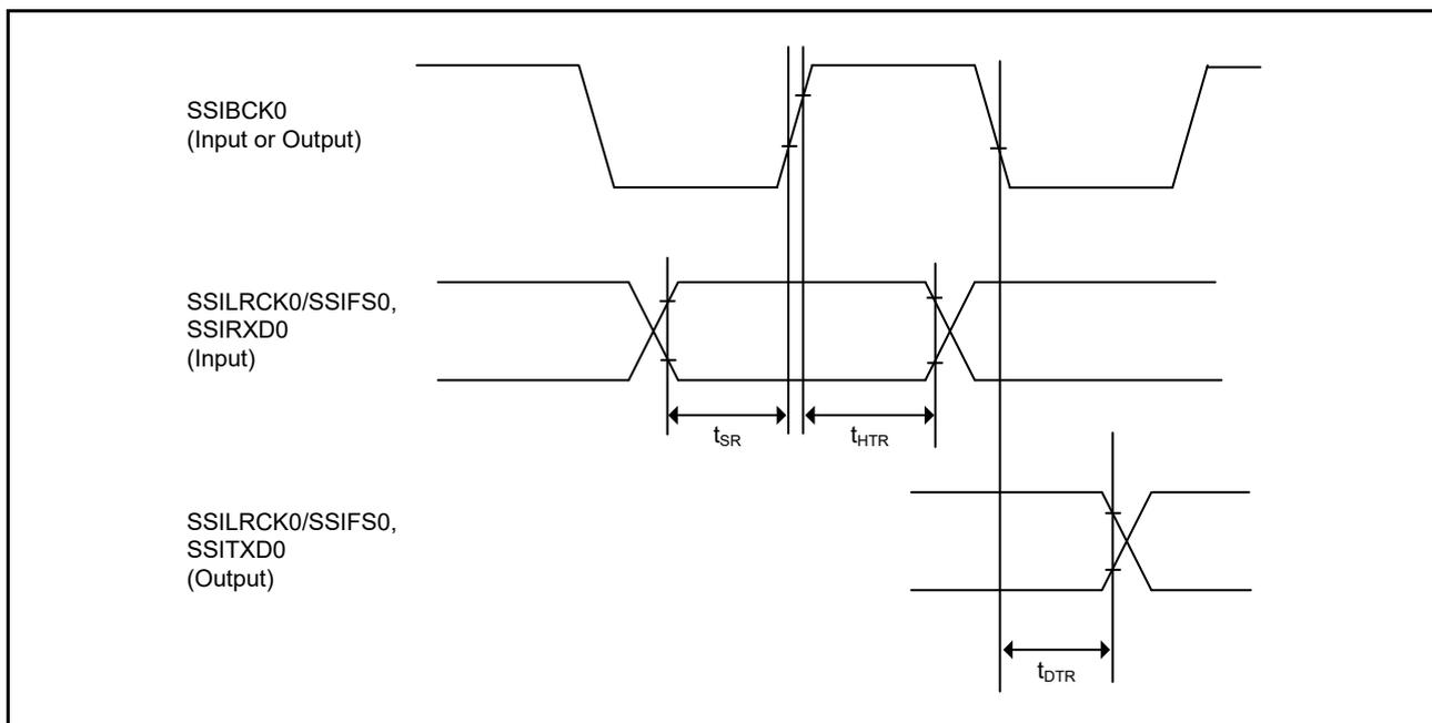
Figure 2.61 SSIE data transmit/receive timing (SSICR.BCKP = 0)
