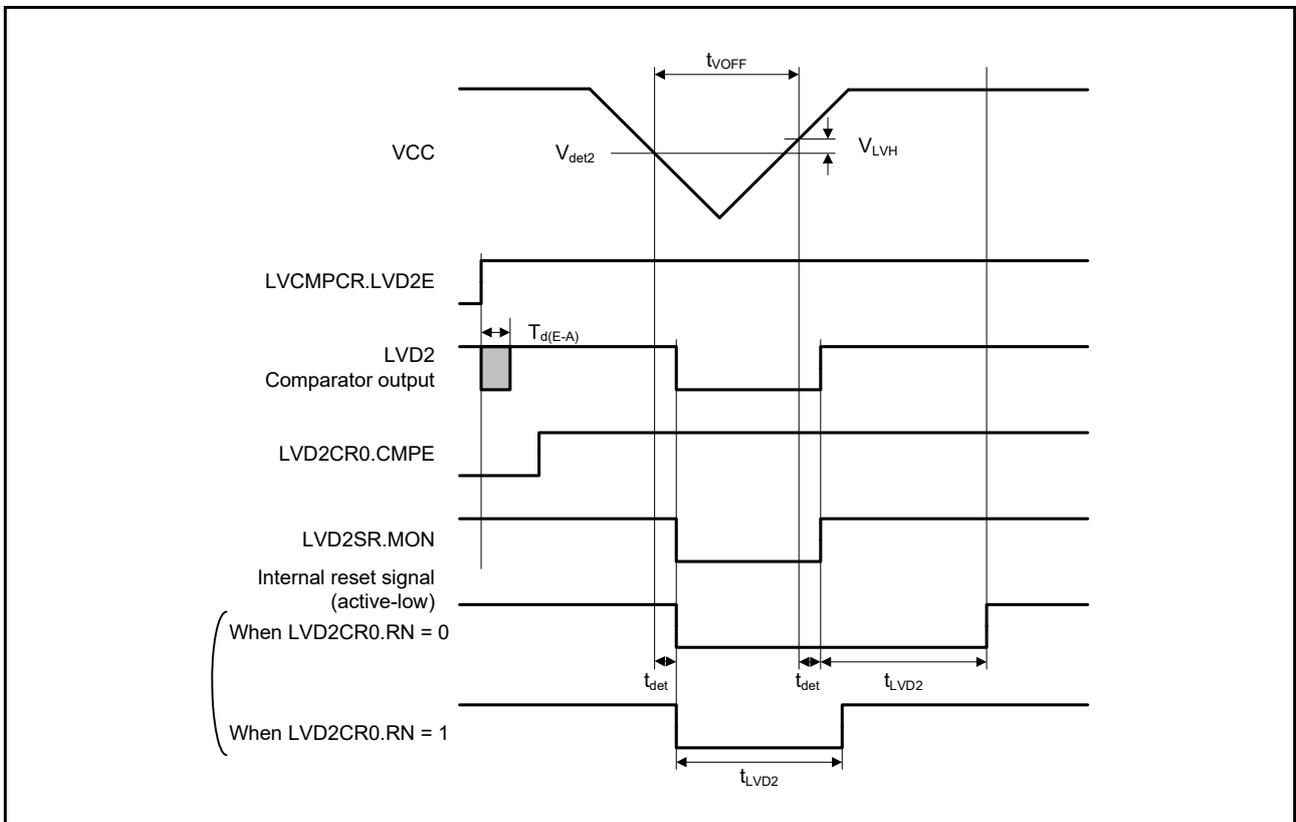
Figure 2.77 Voltage detection circuit timing ( $V_{det2}$ )
